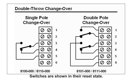
Figure 4a: Wiring Configuration
