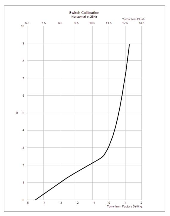
Figure 6: Vibration Switch Calibration Curve.
