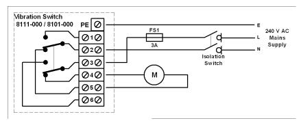
Figure 4b: Typical Installation - Circuit Diagram
