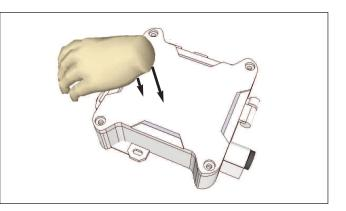
Check lever moves freely up and down.
