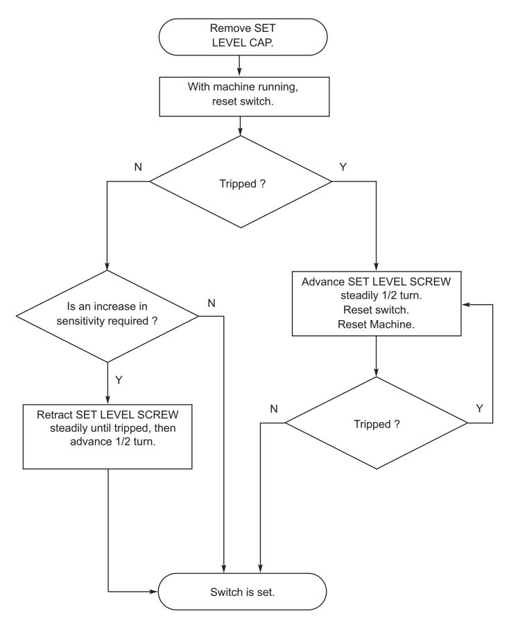
The SET LEVEL can be estimated by referring to the calibration curve in figure 6 and counting the number of turns from the factory setting.
